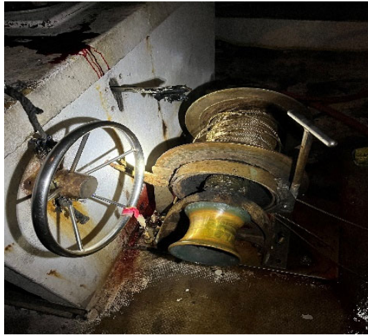
Figure 3. KIM LY winch with no guard - Anne's Bait Shop Ingleside, TX. (February 20, 2024/USCG)
